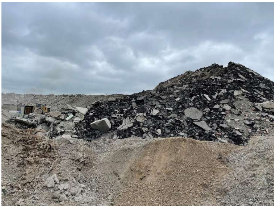
Photo (6): Strada Crusher at 1667 Creditstone Rd, Concord, ON – Old Asphalt Raw Material
