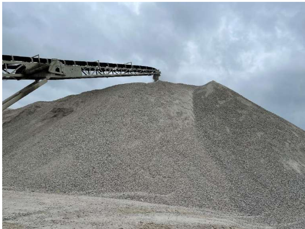
Photo (8): Strada Crusher at 1667 Creditstone Rd, Concord, ON – Stockpile of RCA (Gran A RAP)
