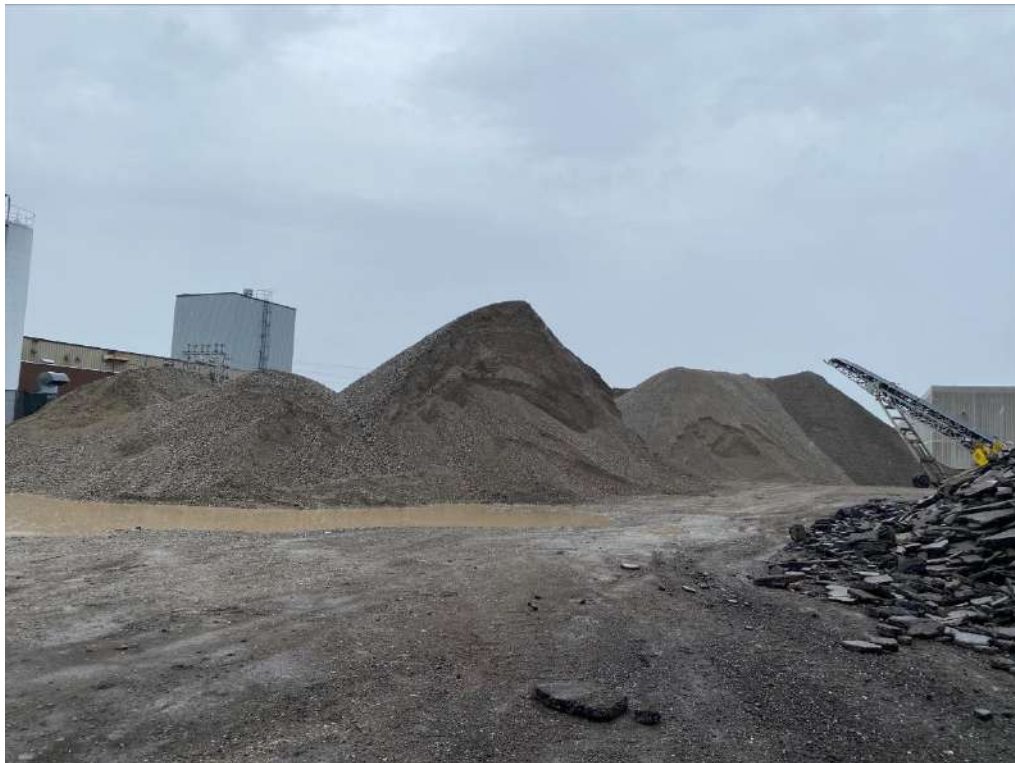
Photo (18): Crupi Crusher at 176 Bethridge Rd, Etobicoke, ON – Stockpiles of RCA
