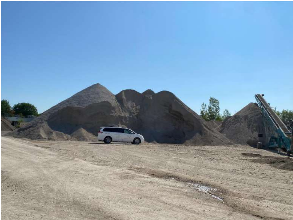
Photo (34): Strada Aggregate Crusher: 10 Leslie St, Toronto, ON Stockpiles of RCA (Gran A Rap) – Sample Collection
