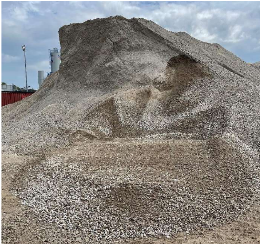
Photo (16): Crupi Crusher at 2777 14th Ave, Markham- Produced RCA (Gran A RAP)
